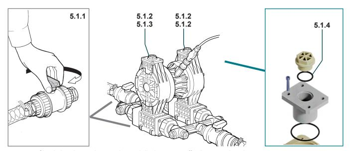
5.1.1 Check that the product suction and discharge cut-off valves are closed.
