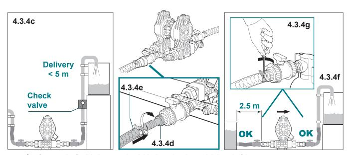
4.3.4f Connect the flexible hoses to the rigids ducts (suction and delivery) of the system.
