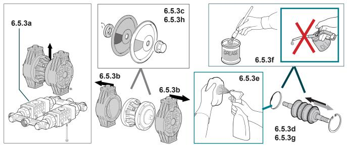
6.5.2e Clean the central and the diaphragms using a disposable clean cloth dampened with a suitable detergent (for the construction material of the pump and the treated product).
