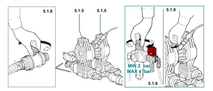
5.1.10 Check that there are no product leaks from the upper plugs of either pump casing. If this is not the case, stop the pump promptly, disconnect the product suction and delivery valves, and re-establish the hydraulic seal before restarting the pump.
