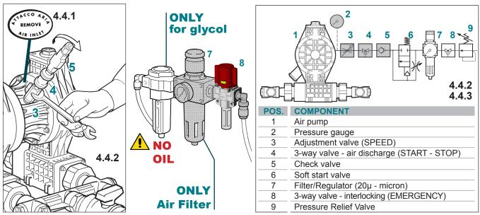
4.4.2 Tighten a compressed air flow control valve, a 3-way valve (START - STOP with air discharge) and a check valve on the pneumatic circuit connection of the pump, as per the diagram in the figure. Install a pressure gauge on the compressed air connection of the pump itself and check the value with the pump running to check the actual pressure of the supply air.
