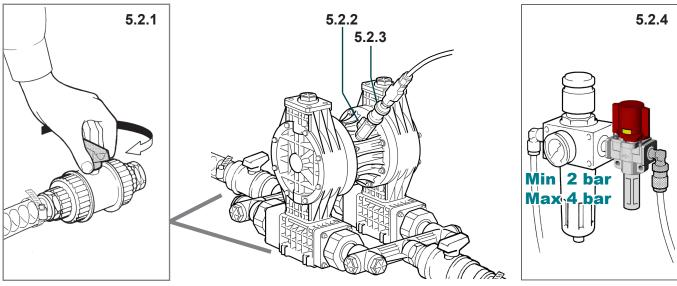
5.2.1 Open the product sectioning valves of the suction and delivery pipes.
