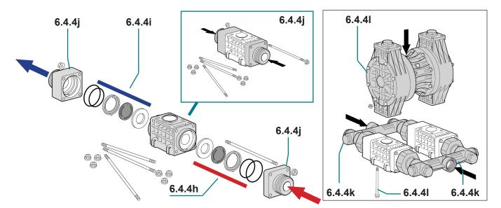
6.4.4l Reassemble the valve bodies on the pump bodies, observing the orientation of the suction and discharge connections (see Spare Parts Table) and secure them with the appropriate screws to a tightening torque of 5 Nm.
