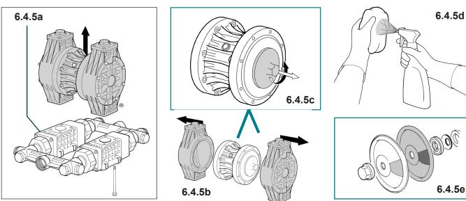
6.4.5a Remove the fixing screws and dismantle the valve bodies with the manifolds of the pumping part.
