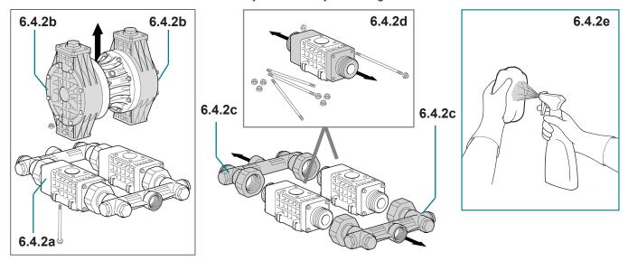
6.4.2d Remove the fixing screws and open the valve bodies.
