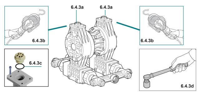
To inspect the pump's diaphragms and clapet valves, proceed as follows:
