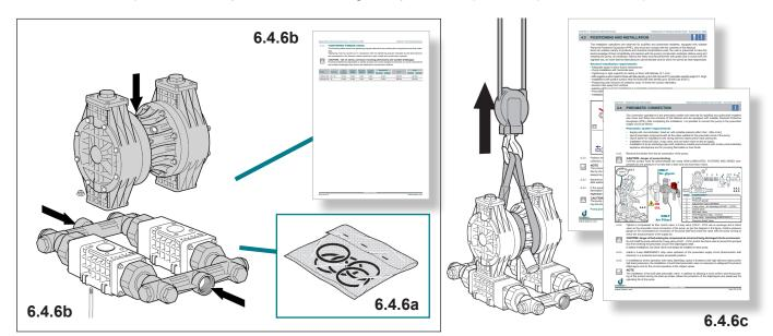
6.4.6b Reassemble the pump in the reverse order to that described above and tighten the fixing bolts progressively and uniformly, observing the tightening torques indicated by the Manufacturer (see 6.3.2 TIGHT-ENING TABLE page 48).
