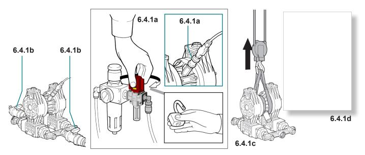
6.4.1a To shut down the pump, only operate on the air supply: close the ball valve and the 3-way sectioning valve. Close and interlock the upstream 3-way safety valve, **discharge the residual pressure from the pump's pneumatic system and fit the safety interlock.**
