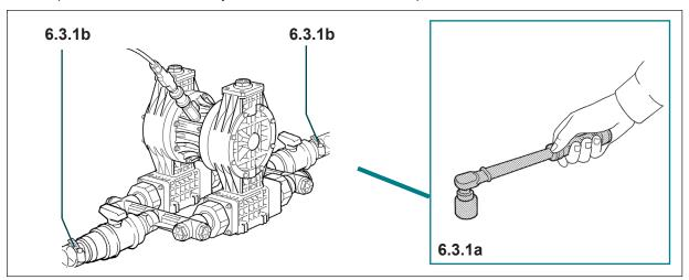
Proceed as follows to check the tightness of the pump:
